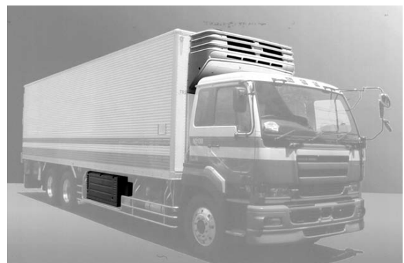
Fig. 12 External view of truck refrigeration unit
