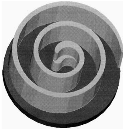
Fig. 10 Profile of new scroll (stepped profile)
