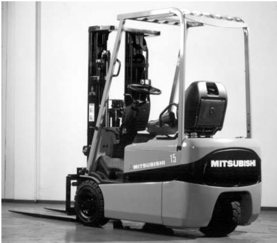
Fig. 8 Rear drive 3-wheel electric counterbalanced forklift truck
