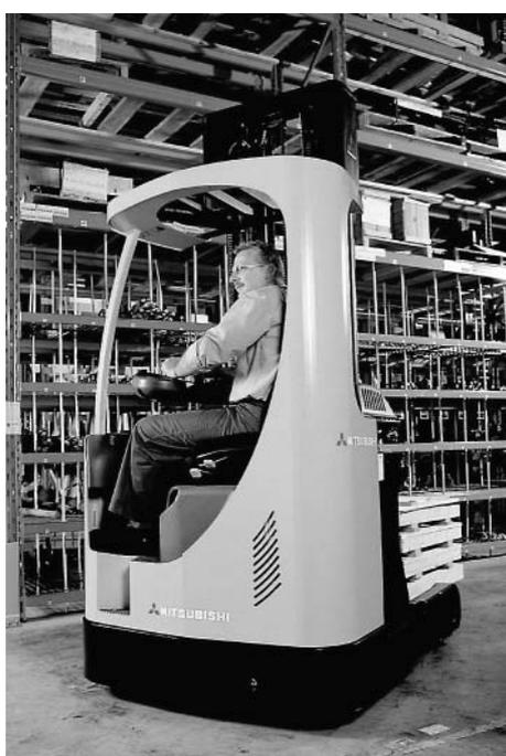
**Fig. 2 Reach type forklift truck**
