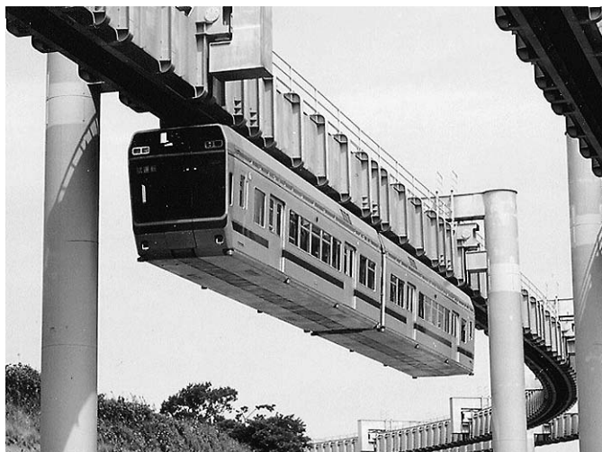
Fig. 1 Suspended monorail "Chiba Urban Monorail"
