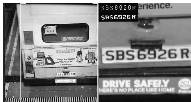
Fig. 7 Vehicle photographed by Singapore ERP and license plate number displayed on monitor
