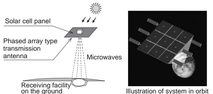
**Fig. 15 Space solar power system (SSPS)**
