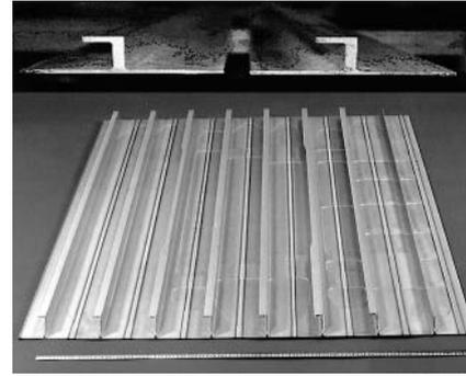
**Fig. 8 View of an integral panel produced by FSW**
