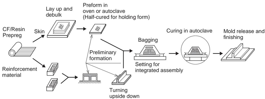
**Fig. 9 Concept of co-cure process**
