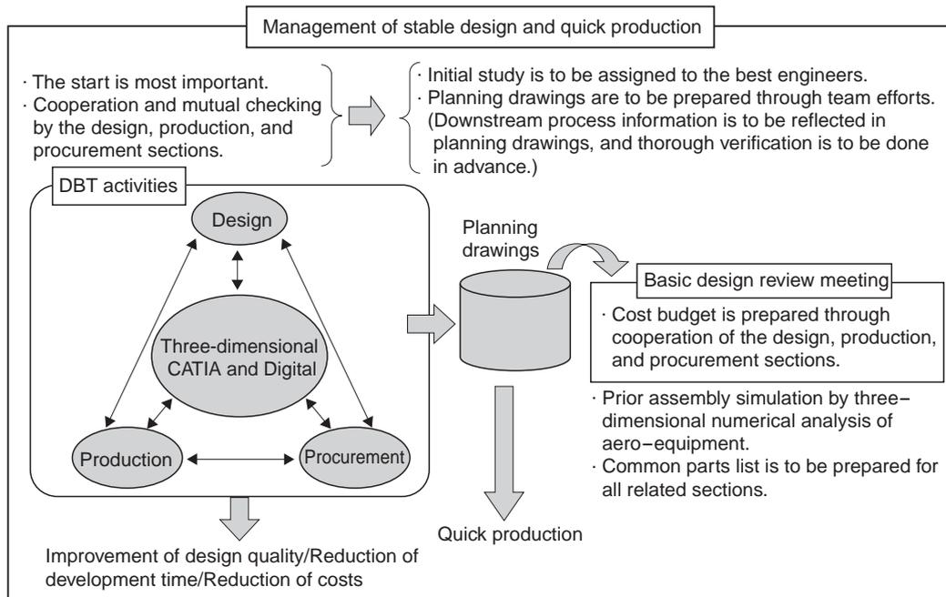
**Fig. 3 Concurrent engineering** The Figure presents an overview of the content of concurrent engineering by cooperation of design, production, and procurement.
