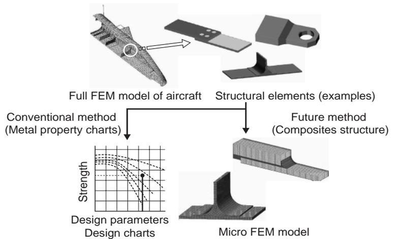
**Fig. 6 Example of structural analysis of composites**
