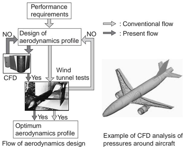
**Fig. 5 Aerodynamic design: CFD analysis**
