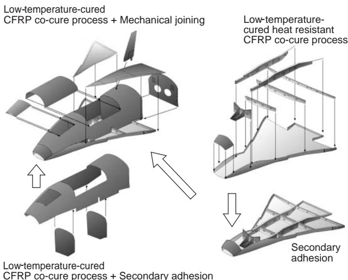
**Fig. 10 Original structure of the prototype of HOPE-X**
