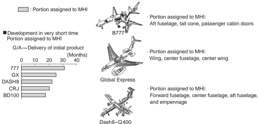
**Fig. 4 Airframe portions assigned to MHI and development period** The Figure shows how development time has been shortened for each aircraft by concurrent engineering.
