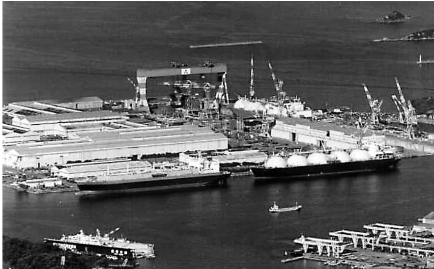
Fig. 1 Bird's-eye view of LNG carriers (spherical tank type and membrane tank type) now being built
