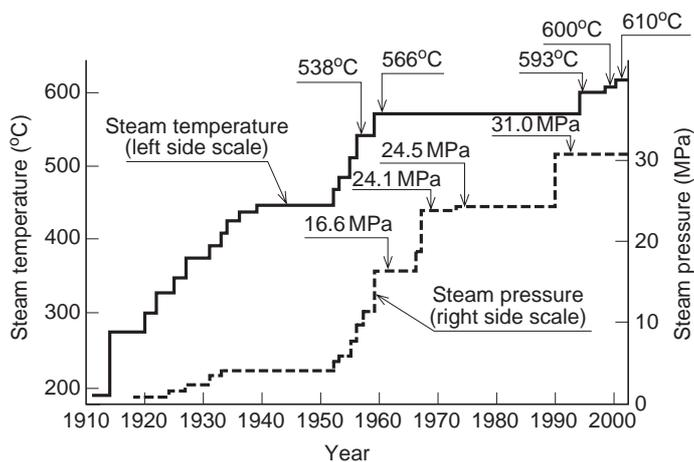
**Fig. 2 Changes in steam conditions of thermal power plants**
