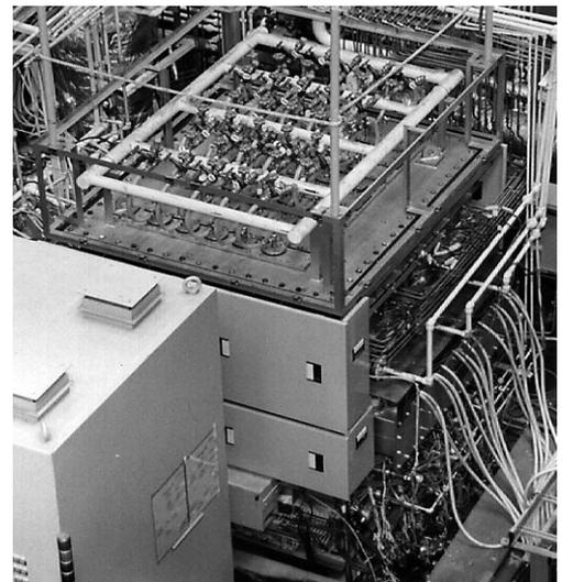
**Fig. 14 MOLB type SOFC atmospheric pressure 10 kW class module**
