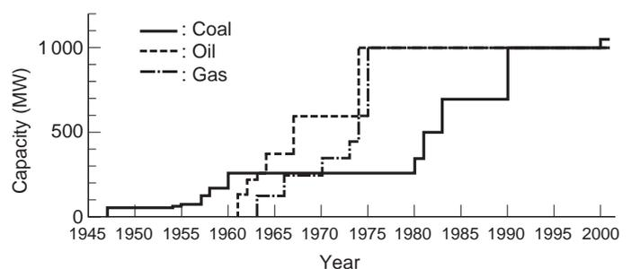
**Fig. 1 Changes in unit capacity of thermal power plants**
