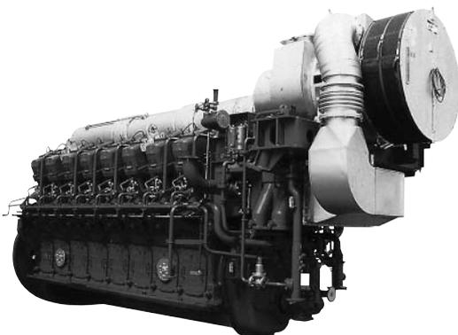
**Fig. 15 Highly efficient gas engine MACH-30G**
