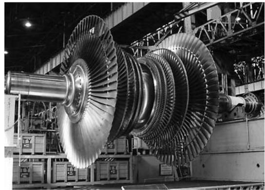
**Fig. 7** Low-pressure turbine using 3 000 rpm 48 inch blades
