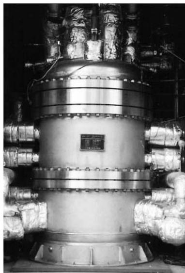
**Fig. 13 Tubular type SOFC pressurized 10 kW class module**
