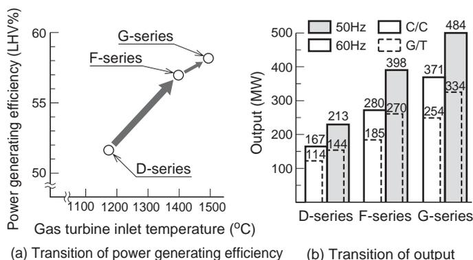
**Fig. 11 Transition of increase in capacity and efficiency of gas turbines**
