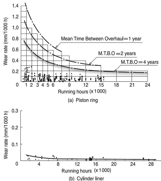
**Fig. 2 Service result of piston ring and cylinder liner wear of UEC-LSII type engine**
