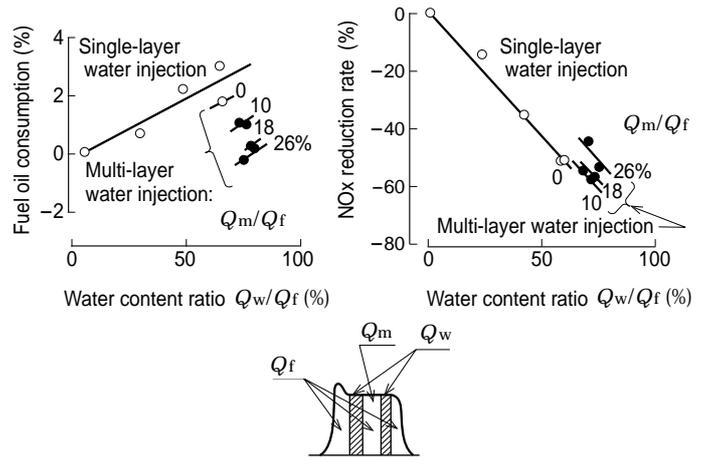
**Fig. 6 NOx reduction rate by the MHI stratified fuel/water system**
