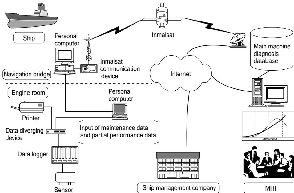
**Fig. 7 Diagnosis system utilizing information technology**
