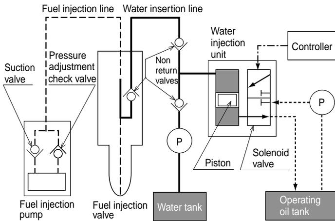
**Fig. 5 Outline of stratified fuel/water injection system**
