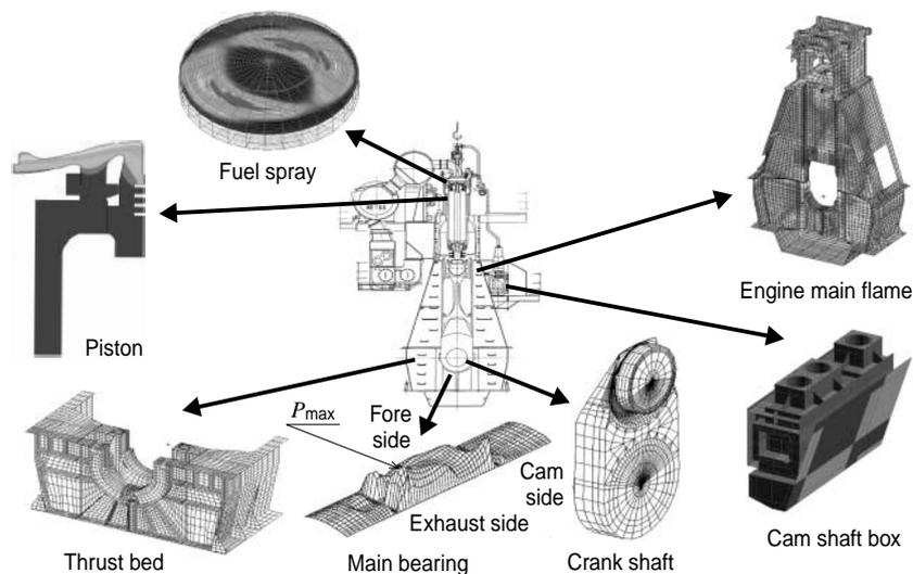
**Fig. 3 CAE application for UEC engine design**
