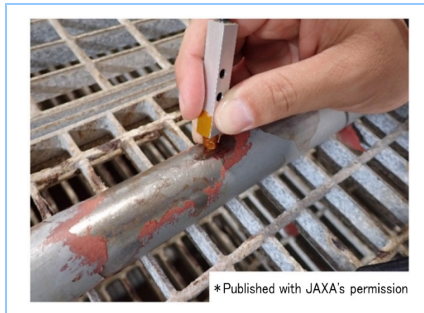
Figure 9 ECT inspection work on outer surface of stainless steel piping
