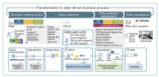
Figure 9 Data-driven service business process with use of remote-monitoring systems
