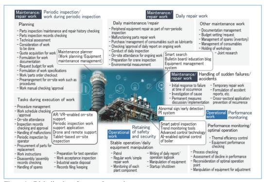
Figure 1 Digitalization of power plant maintenance
