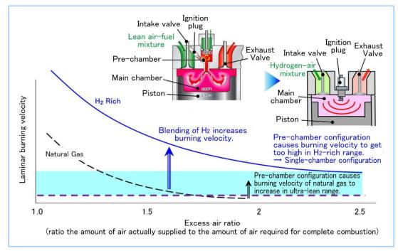
Figure 7 Conceptual diagram of air-to-fuel ratio and laminar burning velocity
