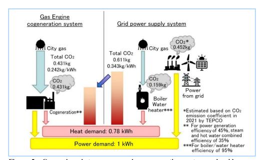
Figure 5 Comparison between gas engine cogeneration system and grid power supply system
