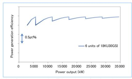
Figure 3 Power generation efficiency with use of multiple units
