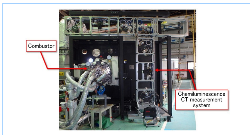
Figure 7 Our atmospheric pressure combustion test rig incorporating chemiluminescence CT measurement system
