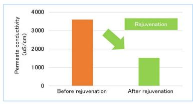
Figure 8 Pilot-scale test result (permeate conductivity)
