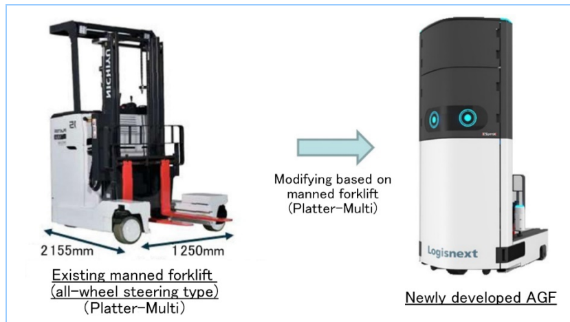
Figure 1 Base forklift and newly developed AGF
