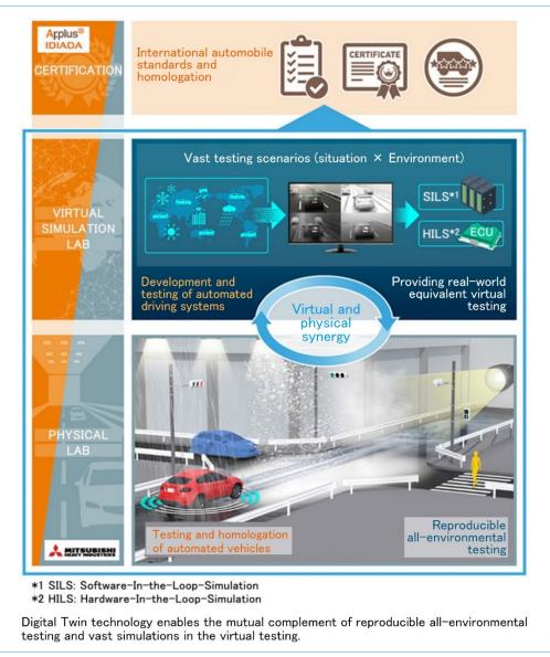
Figure 2 Concept of testing and verification system of advanced automated vehicles and integrated environment testing facility
