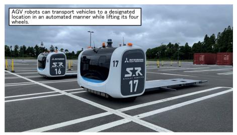
Figure 6 Stanley Robotics AGV car carrying robot "Stan"
