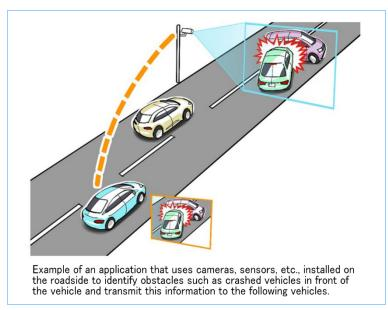
Figure 3 Concept of safety monitoring service
