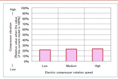
Figure 1 Comparison of compressor vibration between current and new models
