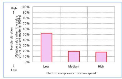
Figure 2 Comparison of handle vibration between current and new models
