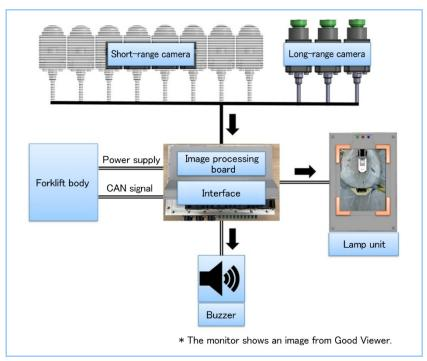
Figure 2 System configuration diagram
