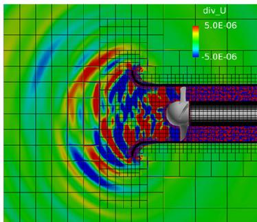
**Figure 4** Example of flow field analysis of axial fan - visualization of aeroacoustic noise propagation
