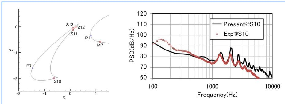
**Figure 3** Example of flow field analysis of aircraft airfoil during take-off/landing - graph of unsteady pressure fluctuation spectrum
