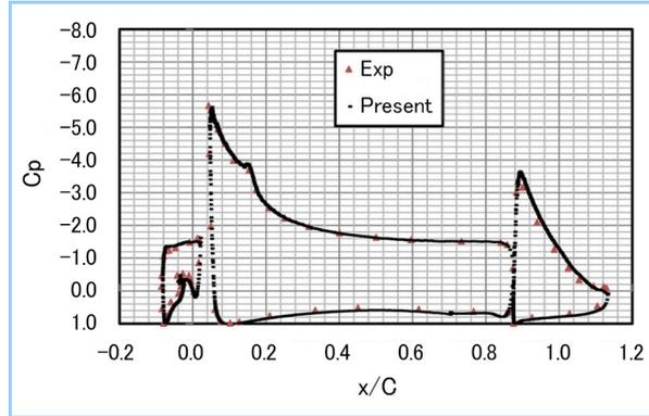
**Figure 2** Example of flow field analysis of aircraft airfoil during take-off/landing - graph of pressure coefficient around airfoil
