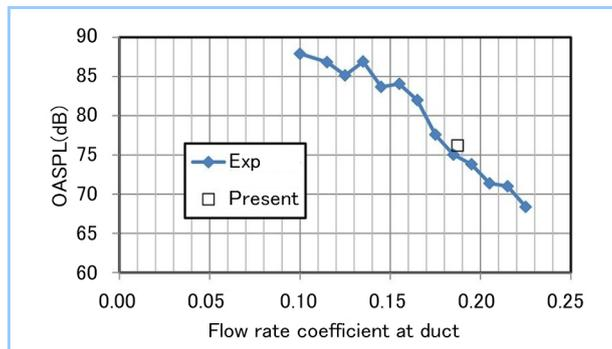
**Figure 5** Example of flow field analysis of axial fan - OASPL graph
