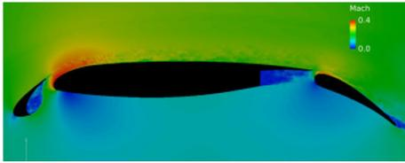
**Figure 1** Example of flow field analysis of aircraft airfoil during take-off/landing - visualization of unsteady flow field
