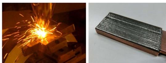
**Figure 13** Results of multi-layer additive manufacturing with copper and ferrous metal
