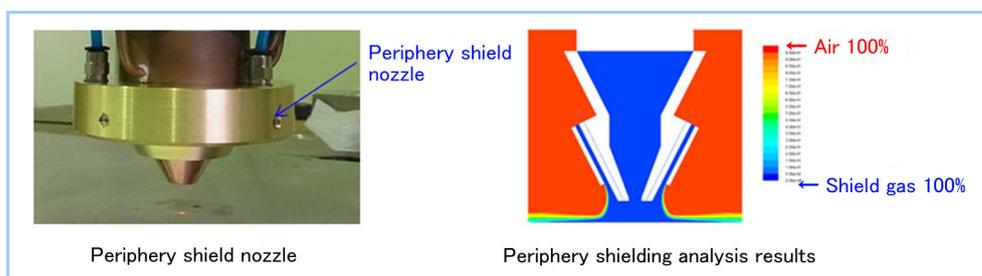
**Figure 7** Periphery shield nozzle and fluid analysis results
