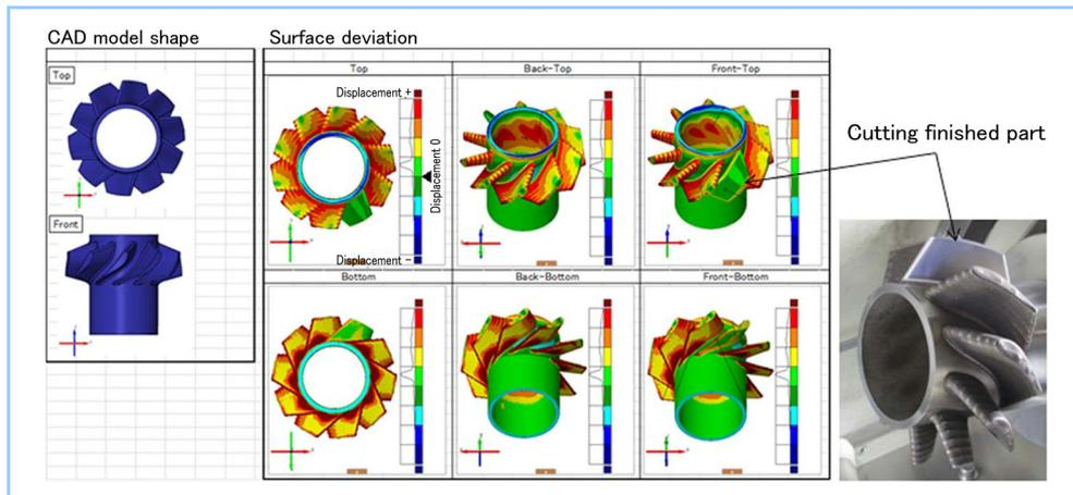
**Figure 10** Evaluation of the additive manufacturing of the blade profile (shape accuracy)
