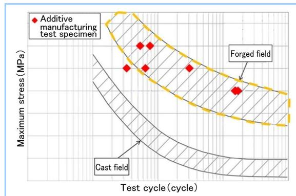
**Figure 12** Measurement results of the fatigue strength of the titanium alloy
