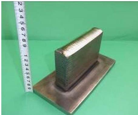
**Figure 11** Titanium alloy specimen for additive manufacturing
