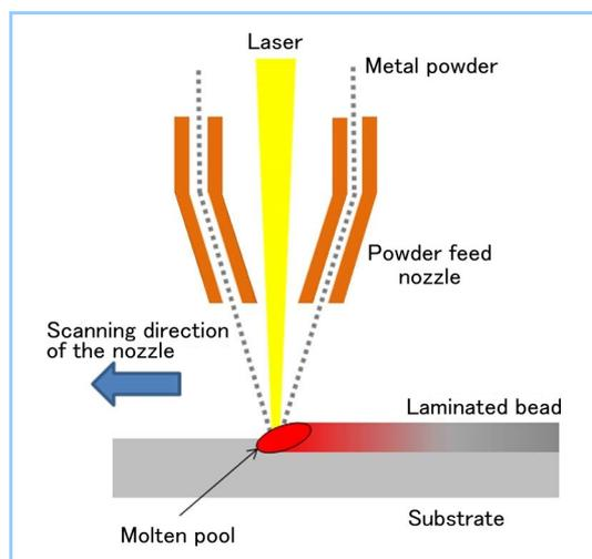
**Figure 1** Deposition-type additive manufacturing method
