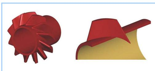
**Figure 8** Shape of the blade profile
