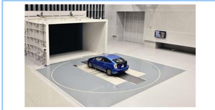
**Figure 4 Full-scale aero-acoustic wind tunnel**
