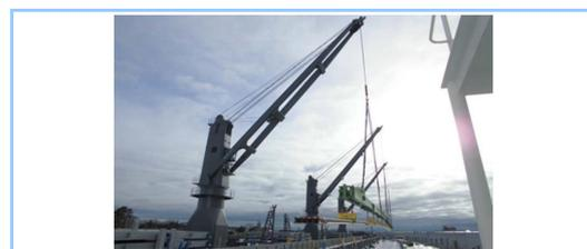
**Figure 3 Deck crane with synchronized control for long rail**
