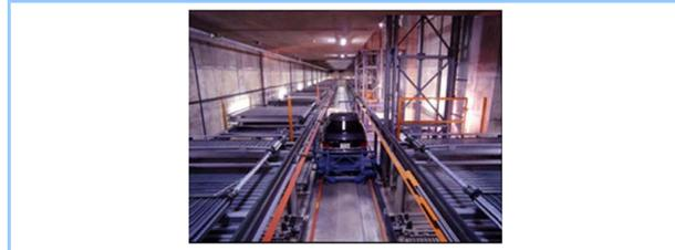
**Figure 5 Integrated parking system (IPS: plane reciprocating/large conveyor type)**
