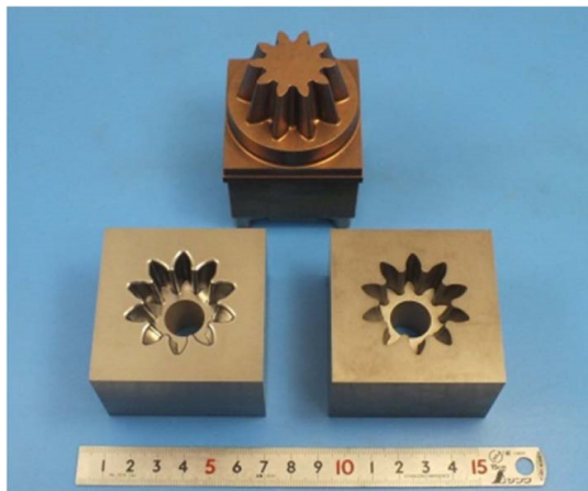
Figure 5 Copper graphite electrode workpiece (above) and bevel gear die (lower left: finished, lower right: unfinished)
