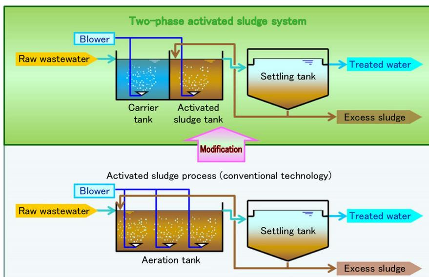
Figure 1 Structure of the two-phase activated sludge system
