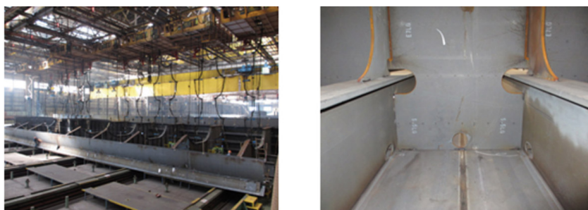
Figure 2 Welding robot application target: Typical example of slot area
