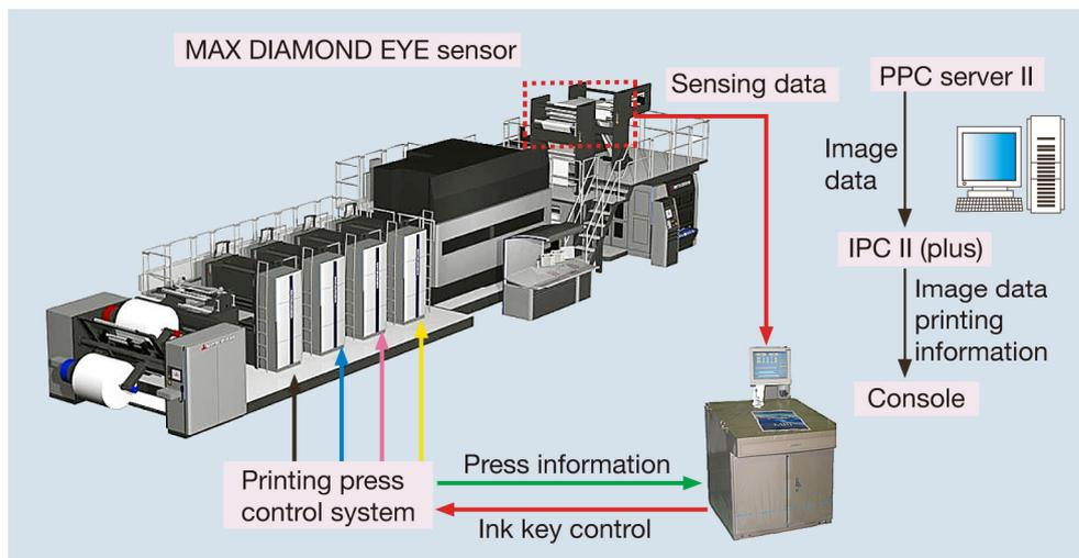
Figure 1 Basic configuration of the MAX DIAMOND EYE in-line quality control system.
