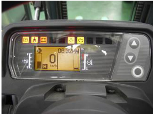
Figure 3 New GRENDiA monitor panel
