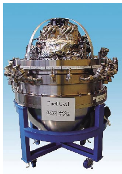
Fig. 7 PEFC installed on Urashima The 4 kW class fully closed loop type was adopted for use in the operational environment of a closed underwater space.
