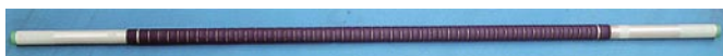
Fig. 3 Appearance of the tubular type cell tube Cell tube of 1500 mm length and 28 mm diameter.
