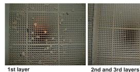
1st layer (uppermost upstream layer) (photo shows the 2nd laver.) Some solidified ash and slight Neither solidified ash nor clogging are observed.
