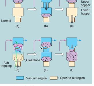
Fig. 13 Lock hopper ash conveying system
