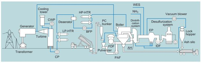
Fig. 6 Schematic of system
