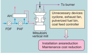
Fig. 3 Direct mill system (direct combustion system)
