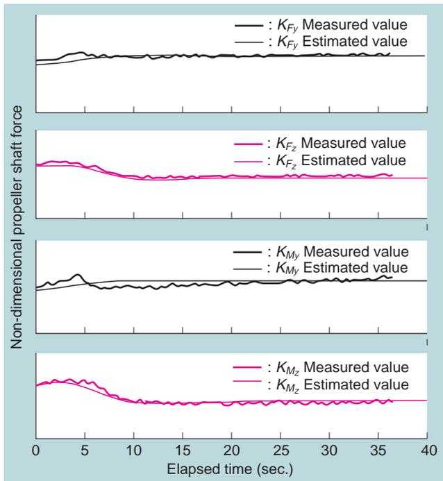
**Fig. 11 Comparison of non-dimensional propeller shaft forces during turning**
