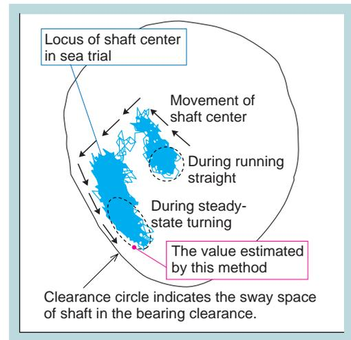
**Fig. 12 Comparison of oil film thickness in stern tube bearing during turning**
