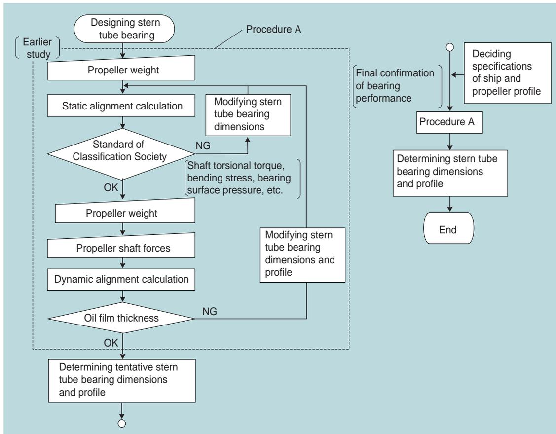
**Fig. 2 Procedure for designing stern tube bearing**
