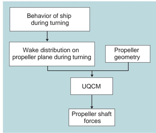
**Fig. 5 Procedure for estimating propeller shaft forces**
