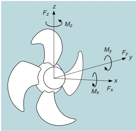
**Fig. 4 Propeller co-ordinate system**
