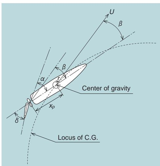
**Fig. 8 Inflow angle into propeller**
