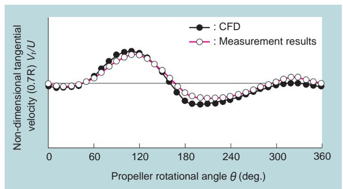
**Fig. 10 Comparison of  $V_t/U$  at representative radius of  $0.7R$**
