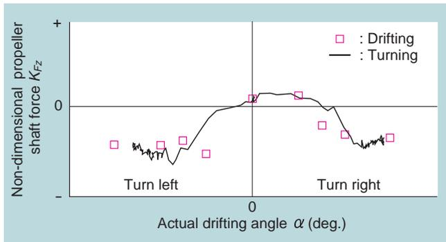
**Fig. 6 Propeller shaft forces during turning and drifting**
