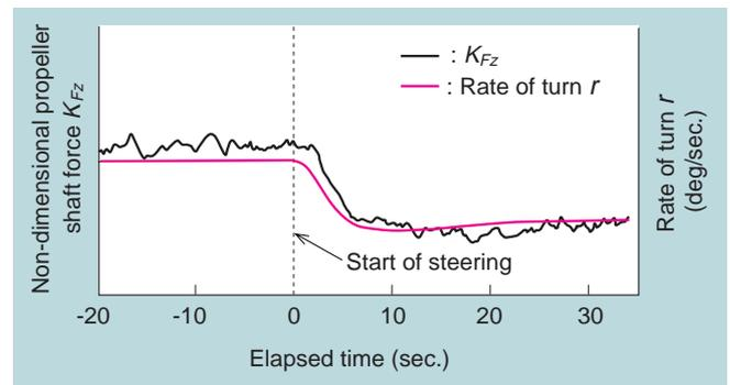
**Fig. 7 Changes in propeller shaft forces during turning**
