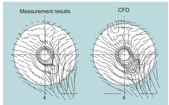
**Fig. 9 Comparison of wake distribution on propeller plane**
