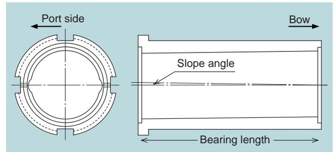
**Fig. 3 Stern tube bearing profile**
