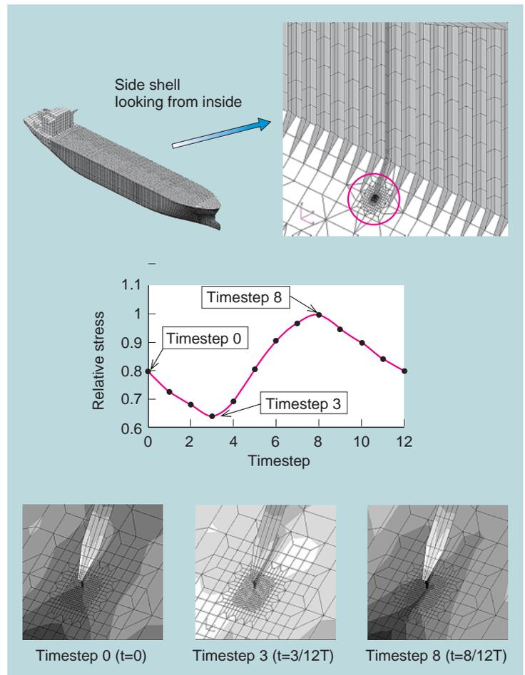
Fig. 3 Simulation of stress response in oceanic waves concerning local stress conducted by DILAM, a sophisticated analysis method
