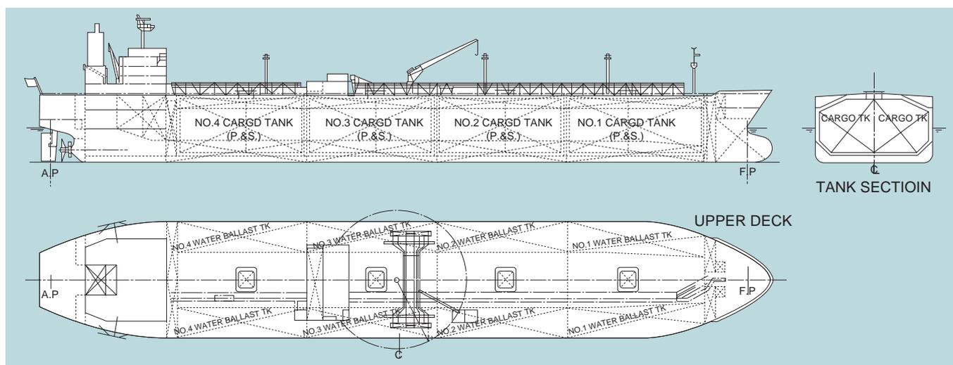
Fig. 1 General arrangement plan
