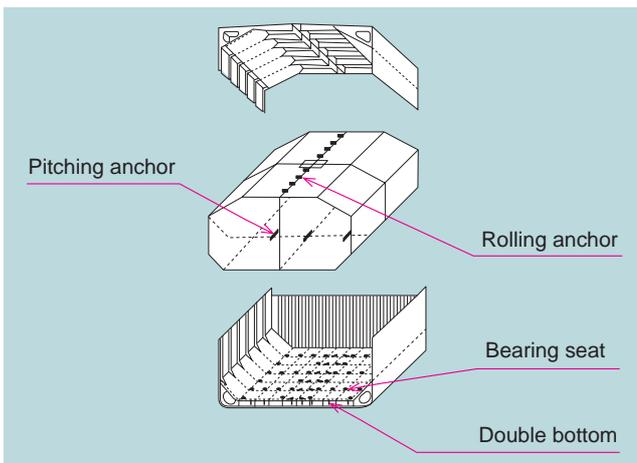
Fig. 2 Tank structure
