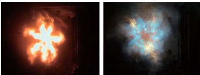
Fig. 10 Combustion of reheat burner at low load
