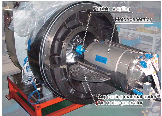
Fig. 5 Hybrid Turbocharger under assembling
