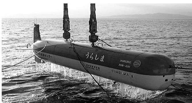
Fig. 1 "Urashima", an autonomous underwater vehicle Achieved the longest continuous cruising distance of 317 km, rewriting the world record for autonomous underwater vehicles powered by PEFC.
