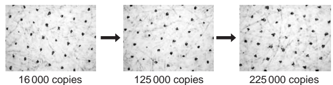
Fig. 5 Halftone dot on paper (5% area) in durability test No dot loss or skip were observed in highlight area showing a first sign of deterioration of print durability.
