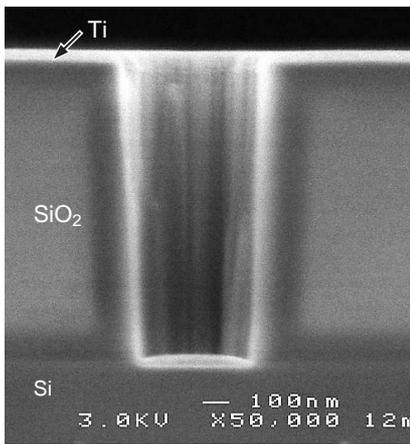
**Fig. 1 SEM photograph of titanium film deposition on a hole pattern**
