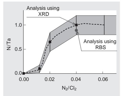
**Fig. 3 Dependence of N/Ta ratio in tantalum nitride film on nitrogen flow rate**
