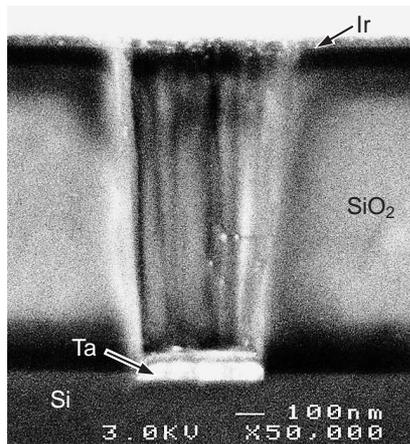
**Fig. 2 SEM photograph of iridium film deposition on a hole pattern**
