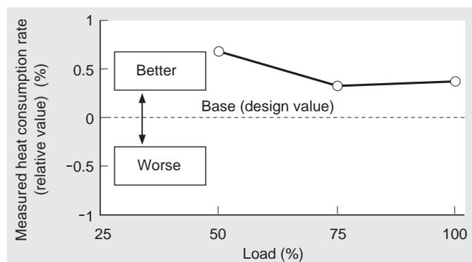
Fig. 3 Turbine performance test results
