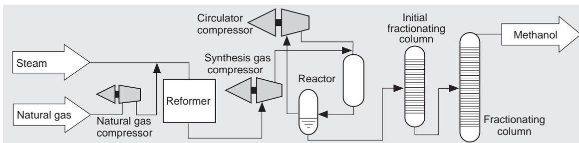
Fig. 2 Configuration of the main equipment in a typical methanol plant
