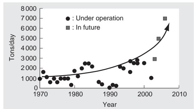
Fig. 1 Overall shift in capacities of methanol plants
