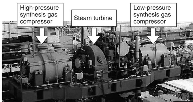
**Fig. 3** Synthesis gas compressor train for a 2 500 tons/day methanol plant (overall length of the equipment is 9.0 m)
