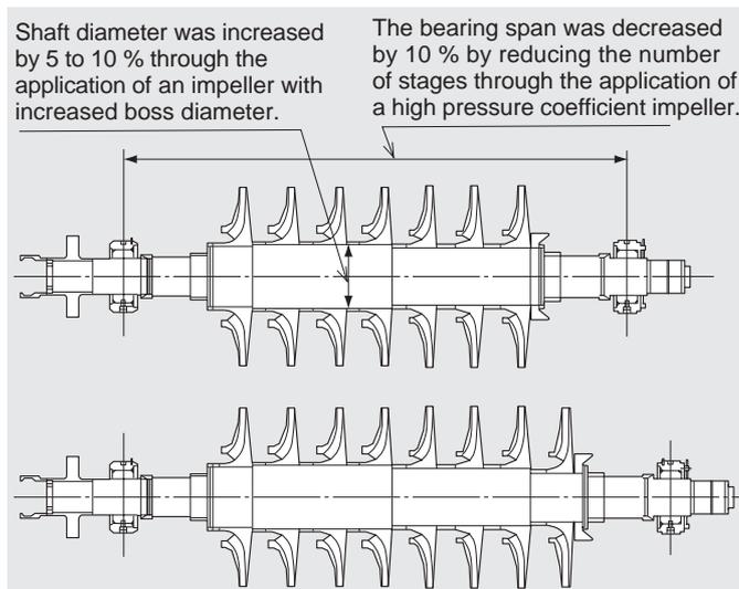
**Fig. 6 Comparison of a rotor to which technologies for increasing capacity have been applied (the upper figure) and a conventional rotor (the lower figure)**
