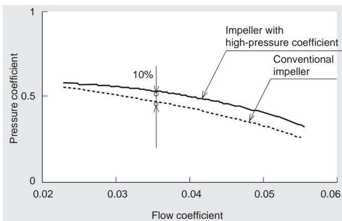
**Fig. 5 Comparison of pressure coefficients between a high pressure coefficient impeller and a conventional impeller**
