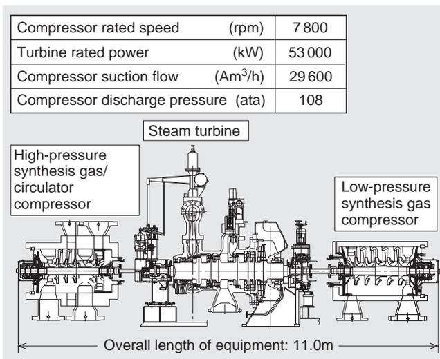
**Fig. 4** Synthesis gas compressor train for a 7 000 tons/day methanol plant
