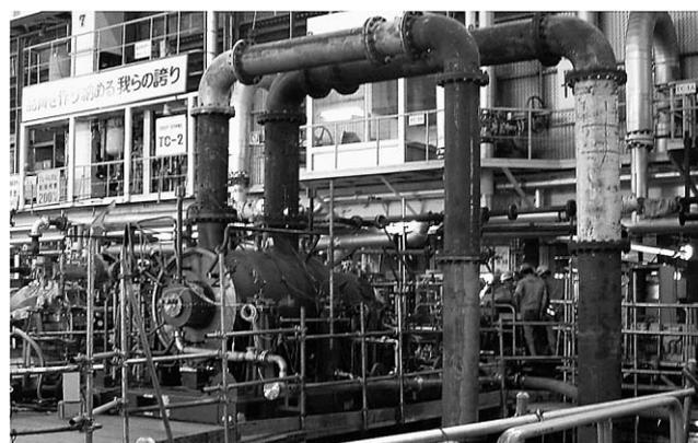
**Fig. 9 Witness test in factory for compressors in a 2 500 tons/day methanol plant**
