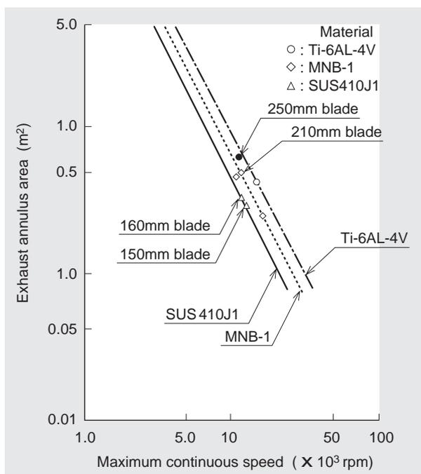
**Fig. 8 Turbine blade for synthesis gas compressor drive**
