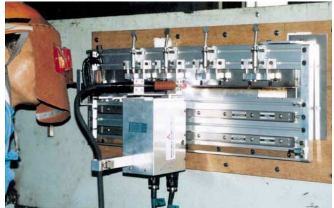
(b) Horizontal position welding
