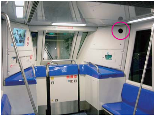
Fig. 11 On-board CCTV camera
