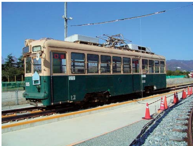
Fig. 6 Test vehicle not using overhead line
