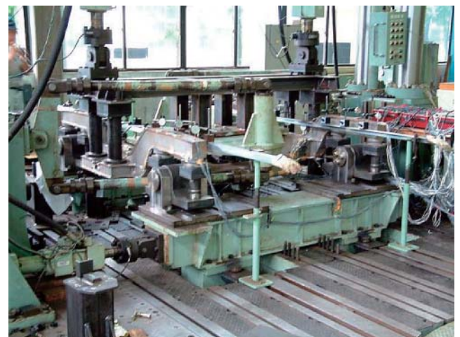
Fig. 4 Static load test of motor-less bogie frame
