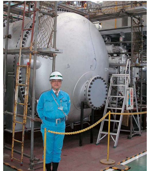
Fig. 7 40 kW class SOFC module The first successful operation in Japan of SOFC gas turbine combined cycle system
