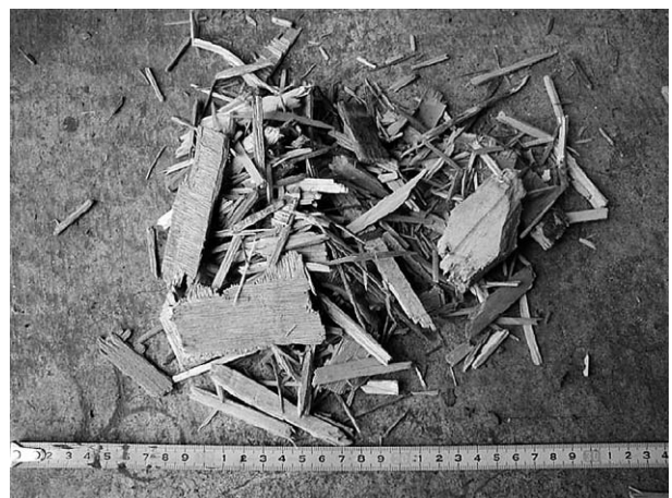
Fig. 2 Appearance of wood products (wood chips) Charging size is about 50 mm or less on longer sides.
