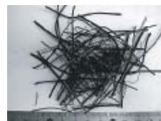
(a) Wires about 60 mm long are recovered by upstream magnetic separator
