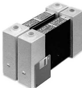
Fig. 8 MOLB type SOFC stack 200 mm x 200 mm power-generation stack made up of active layer, interconnect, gas sealing material, and a manifold.
