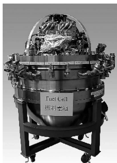
Fig. 2 The PEFC installed onboard the "Urashima"
