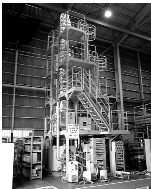
Fig. 4 Test apparatus of continuous PET depolymerization process
