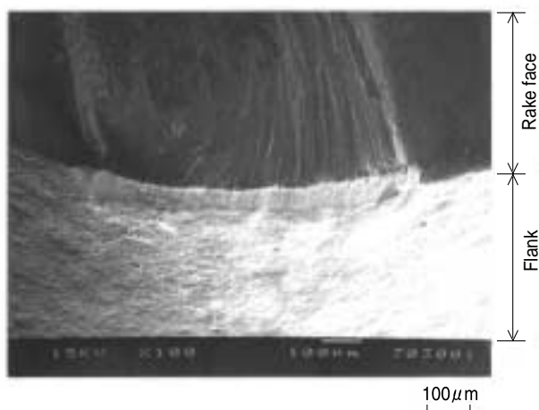
Fig. 1 Tool after cutting 30 m (cutting speed: 30 m/min)
