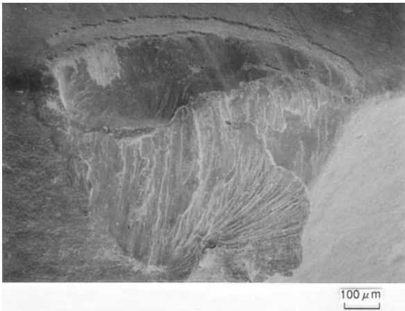
Fig. 4 Tool after cutting 69 m (cutting speed: 100 m/min)
