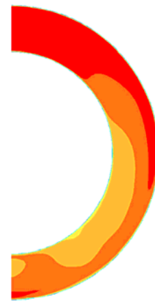
Figure-12 Analysis results of flow velocity distribution at nozzle inlet in new gas inlet casing
