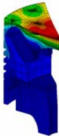
Fig.4 3-dimensional FEM analysis of piston
