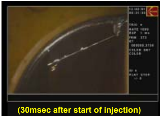
Poor injection due to low temperature
