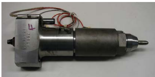
Figure 20. Water injection valve
