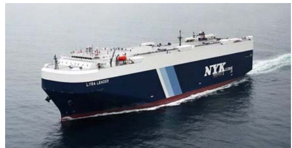
Figure 10. PCTC installed with 8UEC60LSII-Eco
