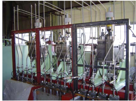
Figure 21. Bench test of independent water injection system
