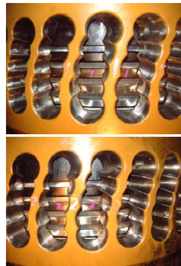
Figure 18. Photos of rings 5755 hours after application of SIP system on UEC50LSII
