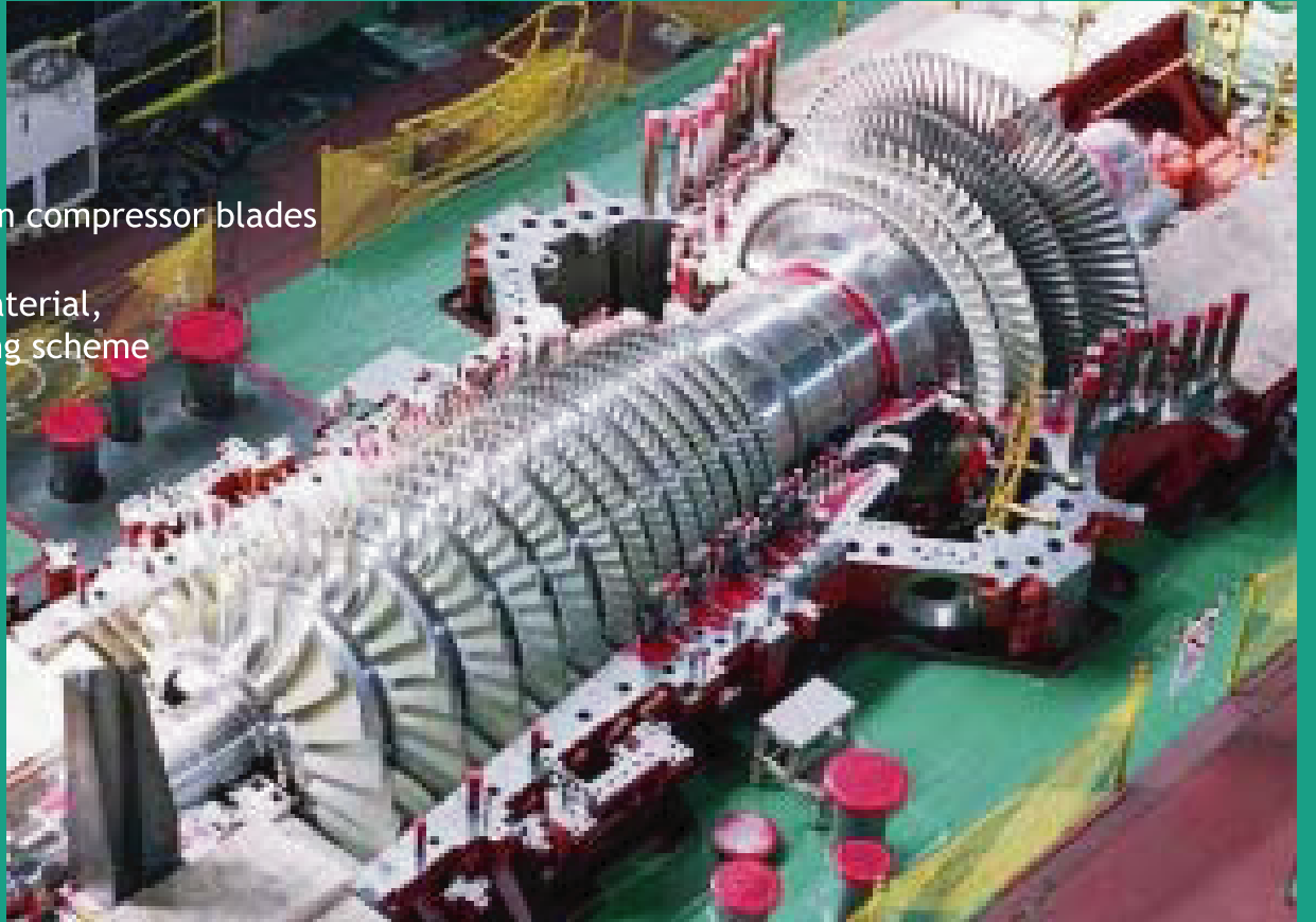
M701G2 : The World Largest gas turbine
